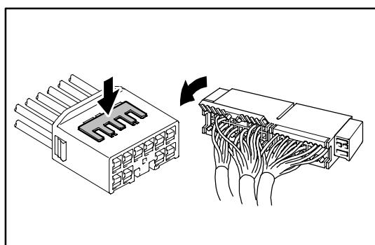
(b) Push the secondary locking device or terminal retainer in to the full lock position.
