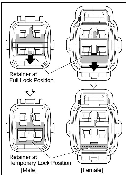
Push the terminal retainer down to the temporary lock position.
